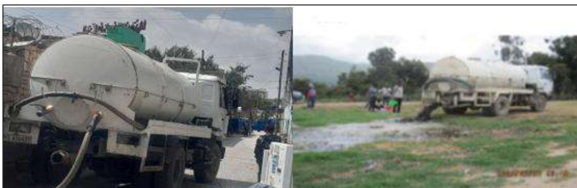
Figure 2.1: Vacuum trucks collecting faecal sludge from pit latrines (left) and uncontrolled faecal sludge disposal in the open field
