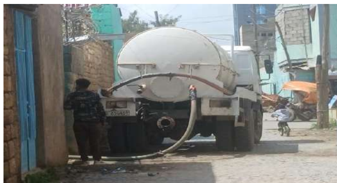
Figure 8.16. Private vacuum trucks collecting faecal sludge from private houses
